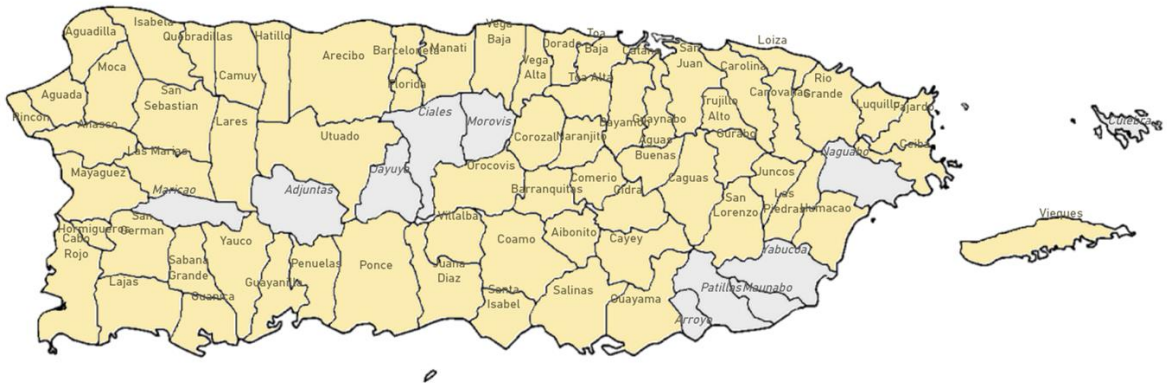
Figure 35 - 16 Municipalities in Grey had 0% Electric Power on December 6, 2017 (Source: M. Castro-Sitiriche, A. Burgos-Rivera, A. Burgos-Cintrón, "Localization of the Communities Reconnected Last to PREPA After Hurricane María: Implications For Hazard Mitigation", PRYSIG 2019, CoHemis, October 25, 2019)
